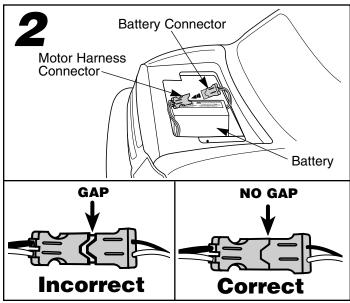
Plug the battery and motor harness connectors together. Push firmly to make sure the two connectors are completely joined.
